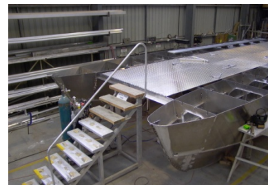
Joining the 2 hulls – 12 m catamaran
